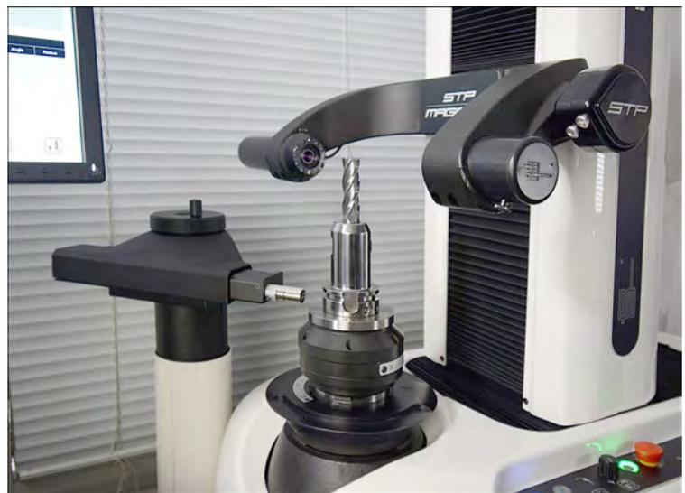
For Pacon, presetting tools offline helps avoid process delays and eliminate errors.
