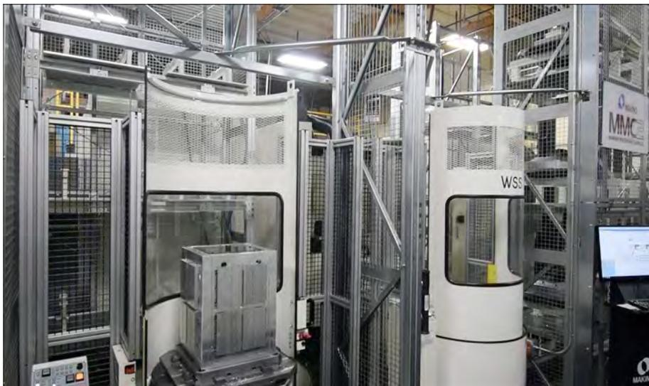
A setup station of a machining cell at Pacon Mfg.
