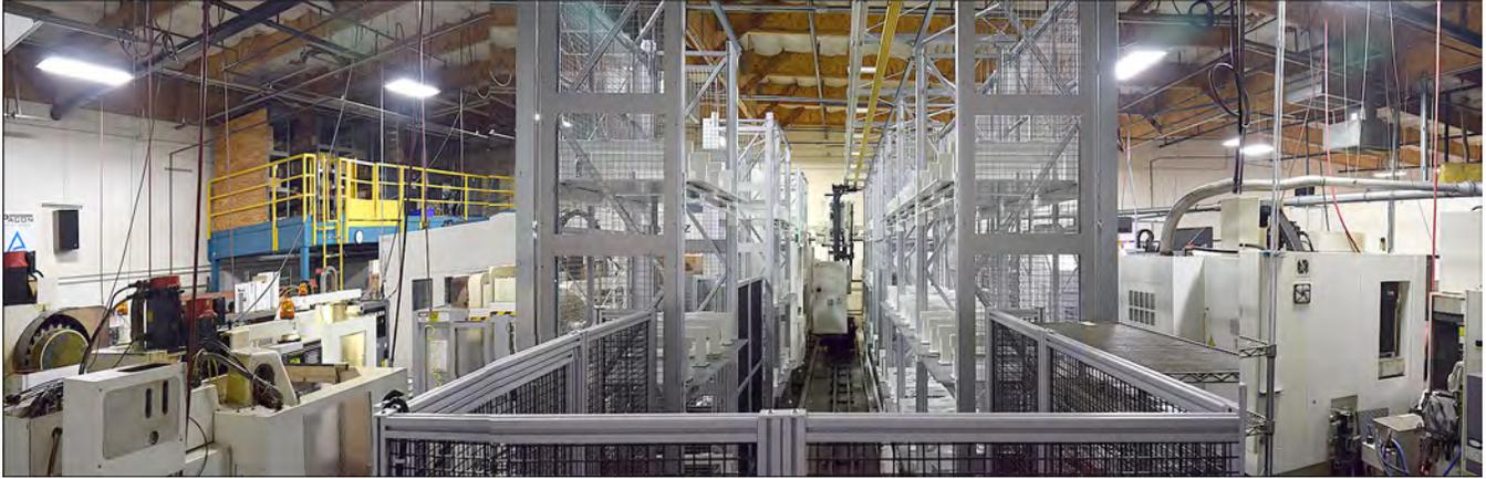
A view down a railway that transfers pallets to two five-axis CNC machining centers.
