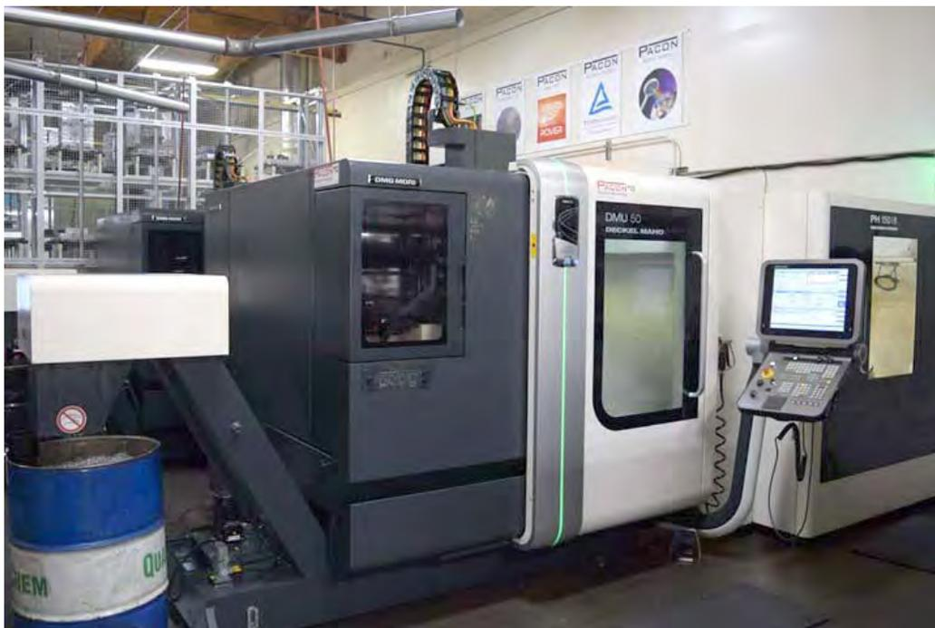
Each of the first two five-axis machines installed at Pacon is serviced by its own pallet pool. All photos: Pacon Mfg, Inc.
